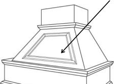
Applied molding on two sides – One side is removable
