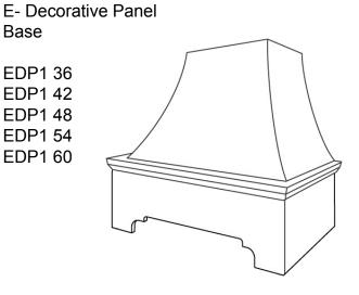
Must Specify height, should not be cut down in the field Call for custom widths / heights
