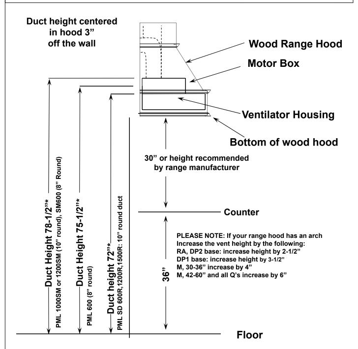
\*Diagram depicts Professional Mesh Liner, increase installed duct heights on the Professional Baffle Liner by 2-3/4"
