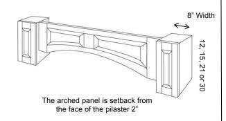
**AV-RPSP Option** – Raised Panel Side Pilasters. Pilasters and valance are sanded to 180 grit ready to finish. Pilasters have a finished bottom. Panel attaches to pilaster with metal brackets and screws (included). Width will be 8" per pilaster. Specify height of pilaster of 12, 15, 21 or 30".
