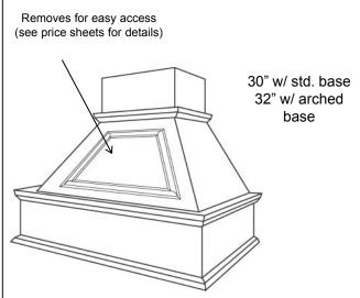
Applied molding – access panel option shown on a standard base G. Order ARP option
